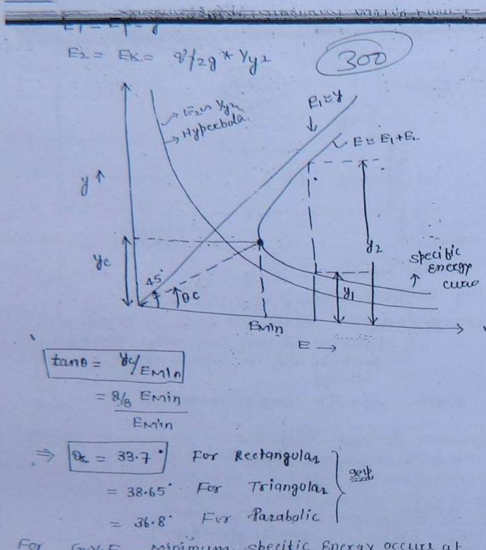
For G.V.F. Minimum specific Energy occurs at which there is only one depth of flow called with depth of Flow (ye). At means at critical flow specific energy is Minimum.
